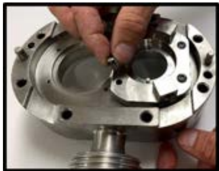
Figure 95 Install seal housing bolts
