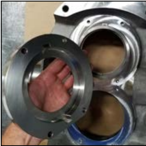
Figure 141 - Install seal housing
