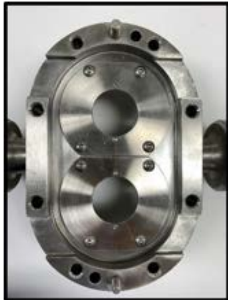
Figure 64 Seal housings installed
