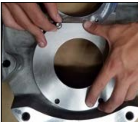
Figure 142 - Install seal housing bolts
