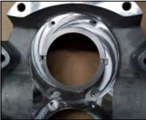
Figure 186 - Drive ring installed
