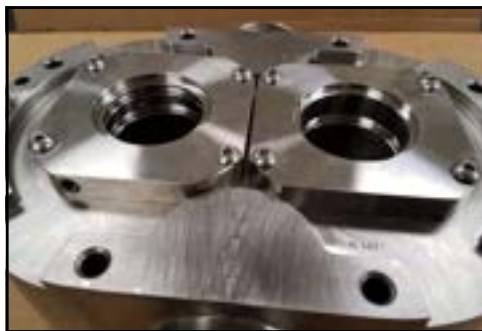
Figure 237 - Seal housings installed
