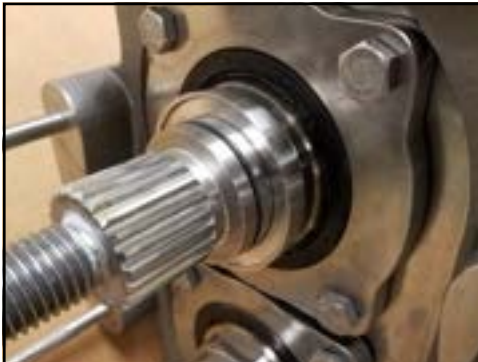
Figure 241 - Seal seat installed
