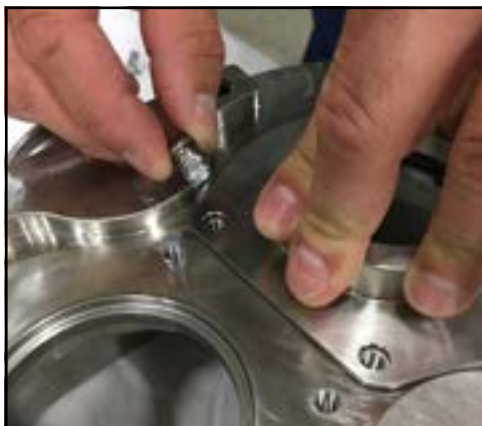
Figure 136 - Install seal housing bolts
