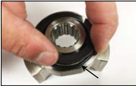
Figure 217 - Seal O-ring pinched
