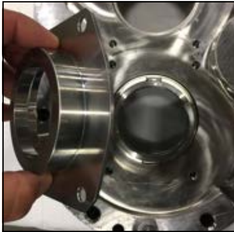
Figure 135 - Install seal housing
