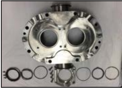
Figure 158 - Double Mechanical Seal (040-U3 shown)
