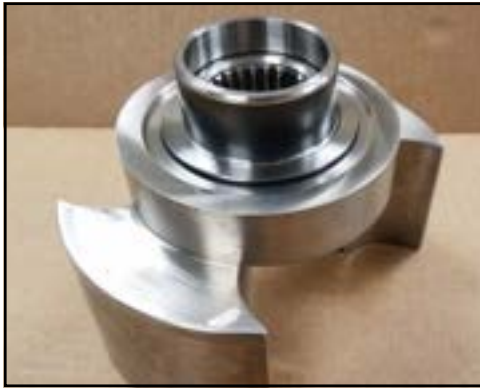
Figure 251 - Seal sleeve installed
