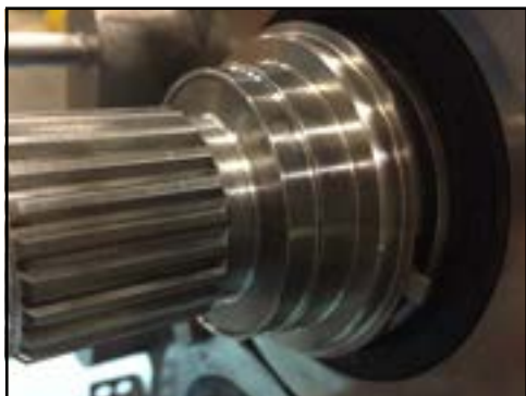
Figure 180 - Adjusting ring installed
