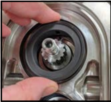
Figure 49 Push stationary seal
