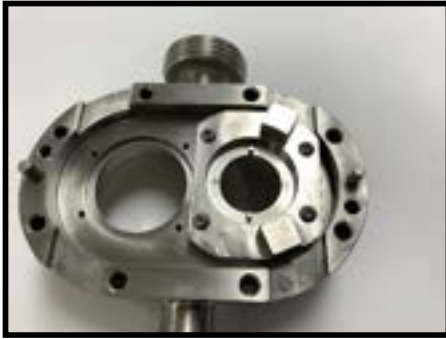
Figure 96 Seal housing installed
