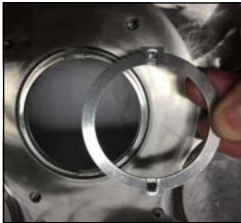
Figure 126 - Remove drive ring
