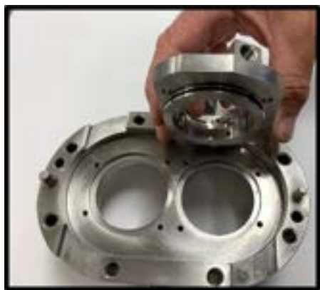
Figure 94 Install seal housing
