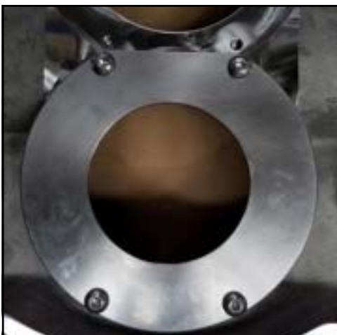
Figure 143 - Seal housing installed
