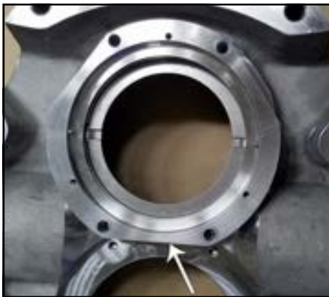
Figure 189 - Seal housing in place
