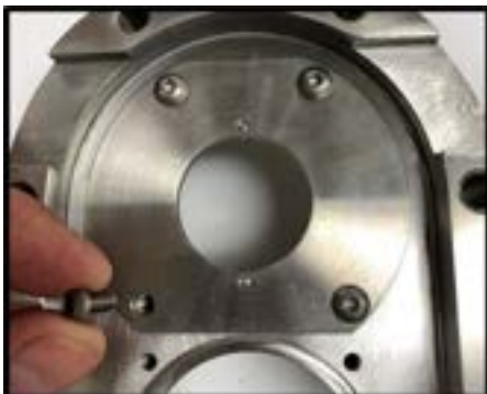
Figure 63 Install seal housing bolts
