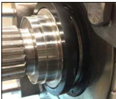
Figure 184 - Rotary seal installed
