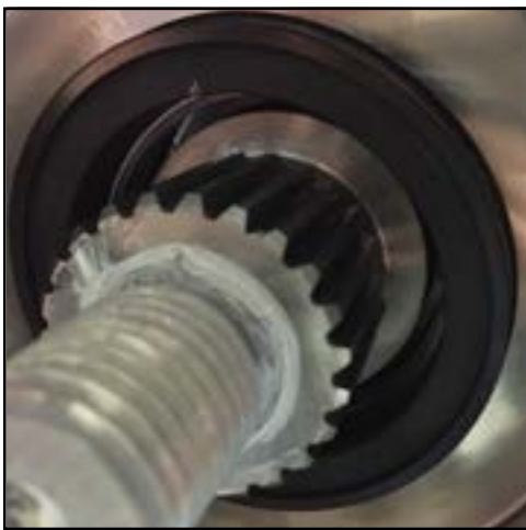
Figure 212 - Stationary seal installed
