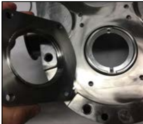
Figure 165 - Install seal housing
