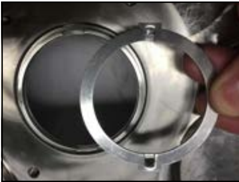
Figure 156 - Remove drive ring
