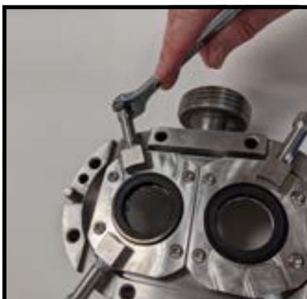
Figure 101 Installing flush port extensions
