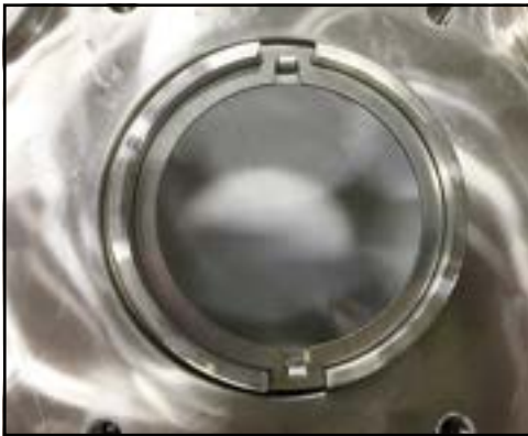
Figure 162 - Drive ring installed
