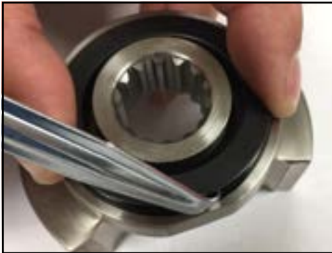
Figure 218 - Push in O-ring
