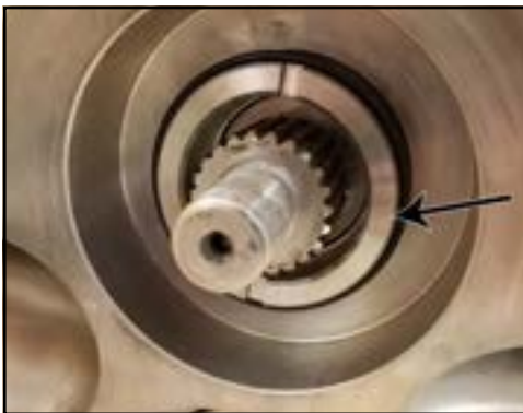
Figure 219 - Sleeve remaining after rotor removal
