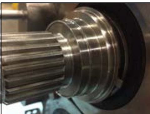
Figure 200 - Adjusting ring installed
