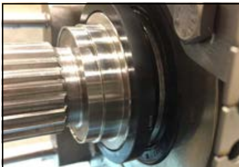
Figure 204 - Rotary seal installed
