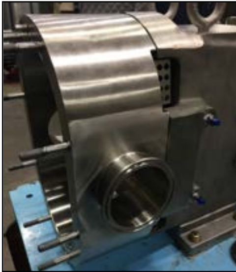
Figure 244 - Pump body installed
