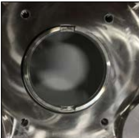
Figure 160 - Shaft ring installed
