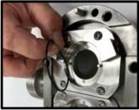
Figure 87 Remove stationary seal O-ring
