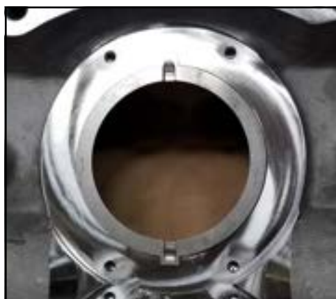
Figure 139 - Drive ring installed
