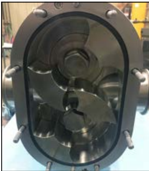
Figure 263 - Cover gasket installed
