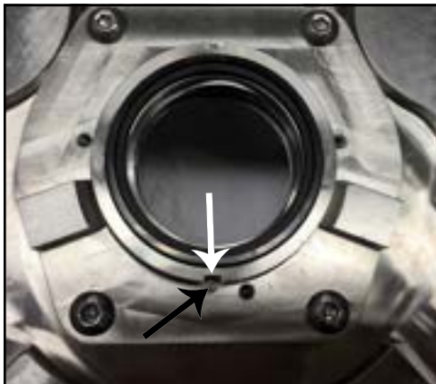
Figure 173 - Flush-side stationary seal installed
