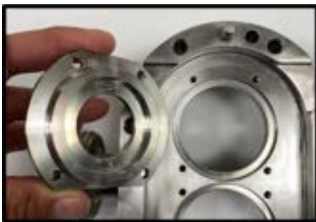
Figure 62 Install seal housing
