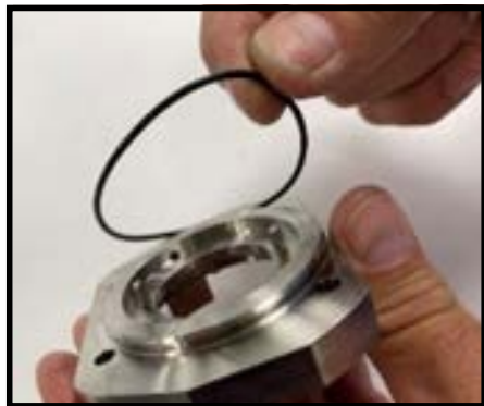
Figure 91 Double Mechanical Seal
