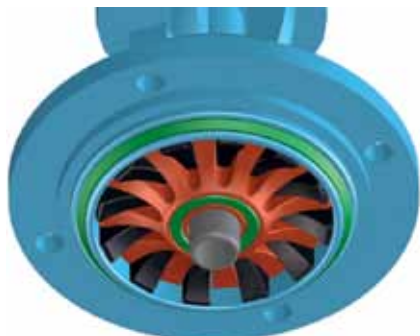
Fan in middle position (valve 50% open)
