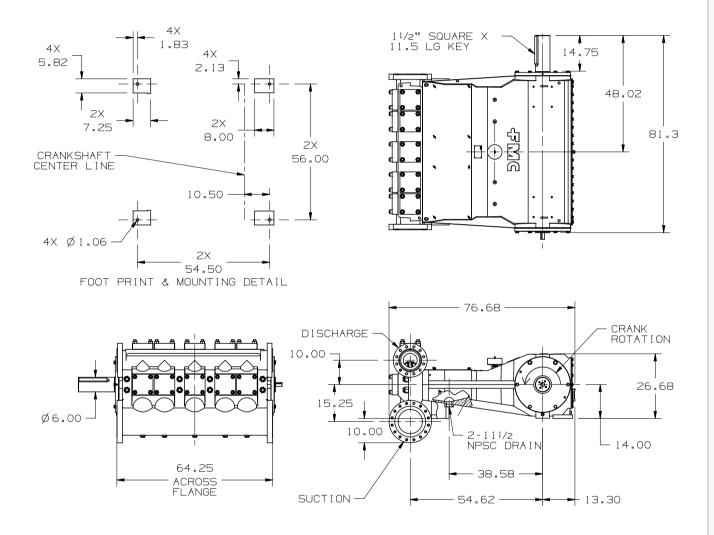
• Dimensions shown are for general sizing purposes and should not be used of construction. Contact FMC for actual dimensions of pump ordered.
