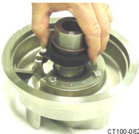
Figure 26 - Push Rotary Seal Down
