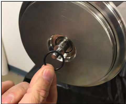
Figure 105 - Install stub shaft O-ring
