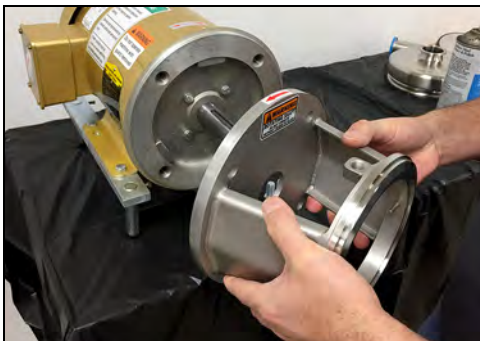
Figure 75 - Remove motor adapter
