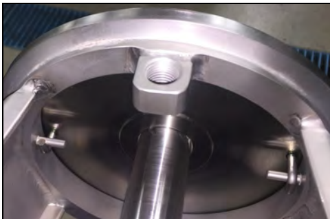
Figure 32 - Backplate pins engaged with adapter pins
