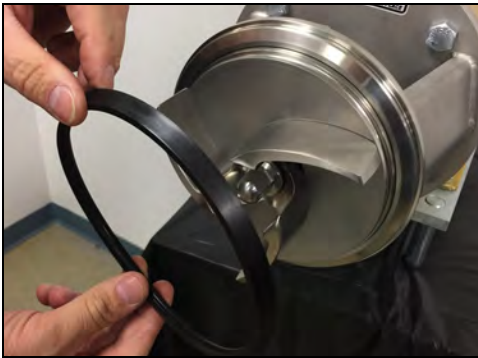
Figure 112 - Place casing gasket onto backplate
