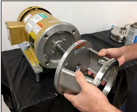
Figure 26 - Remove motor adapter
