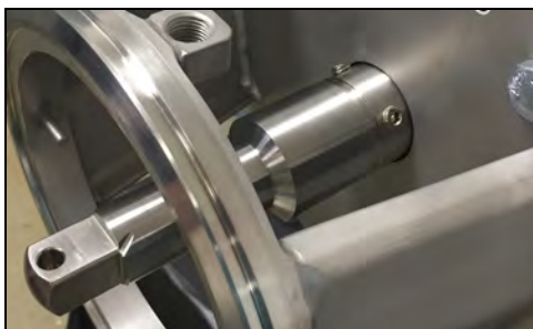
Figure 30 - Stub shaft on motor shaft
