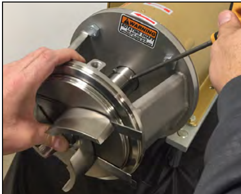
Figure 37 - Place feeler gauge, tighten setscrews
