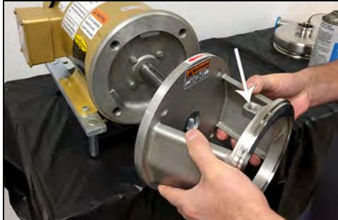
Figure 27 - Install motor adapter
