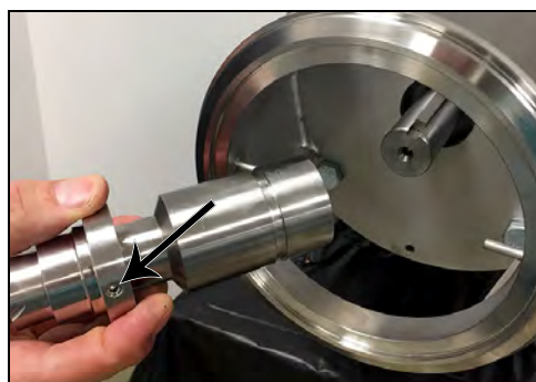
Figure 24 - Pin Impeller: Slide stub shaft off motor shaft
