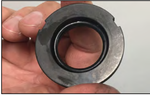
Figure 43 - Seal O-ring installed
