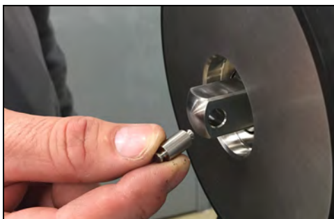
Figure 16 - Remove impeller pin
