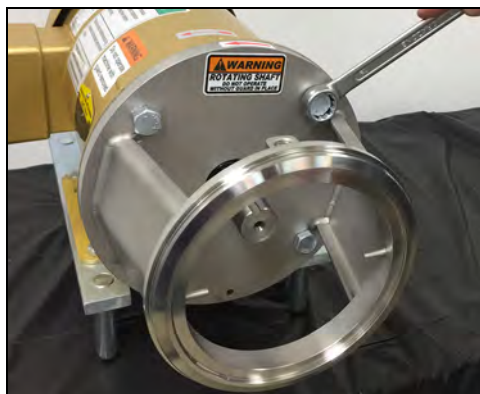
Figure 78 - Install motor adapter bolts
