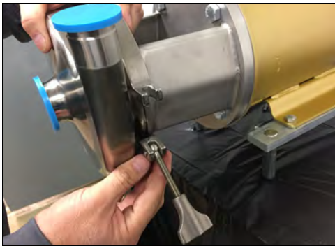
Figure 56 - Remove casing clamp
