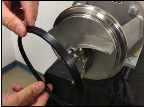
Figure 59 - Remove casing gasket
