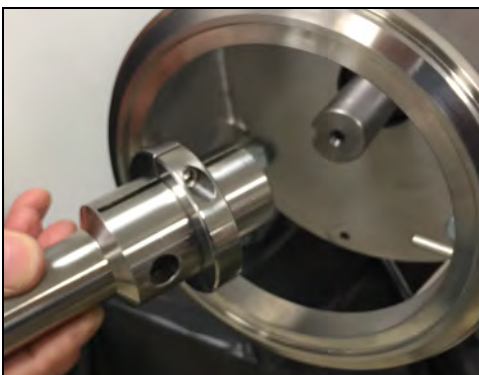
Figure 82 - Slide stub shaft on motor shaft
