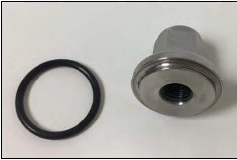
Figure 108 - Install O-ring on impeller nut
