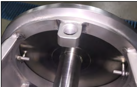
Figure 48 - Backplate pins engaged
