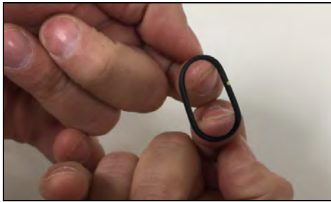
Figure 104 - Lightly stretch O-ring
