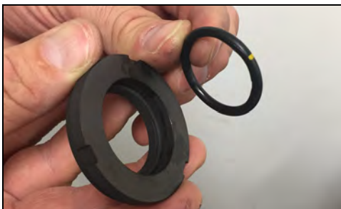
Figure 42 - Lubricate and install O-ring
