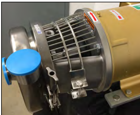
Figure 54 - Install guard assembly
