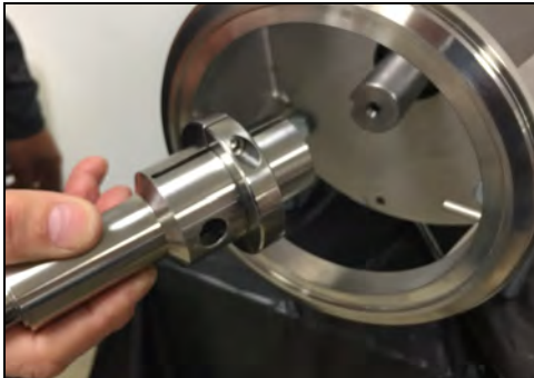
Figure 73 - Slide stub shaft off motor shaft
