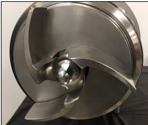
Figure 110 - Hand-tighten impeller nut
