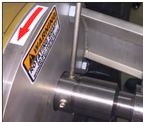
Figure 23 - Pin Impeller: Loosen setscrews
