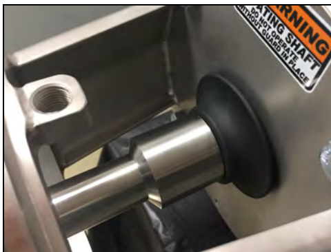
Figure 38 - Slide deflector onto shaft
