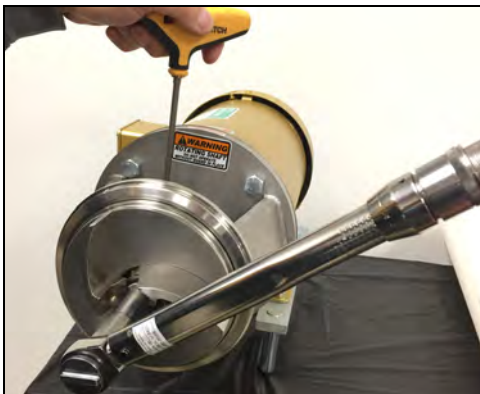
Figure 111 - Torque impeller nut
