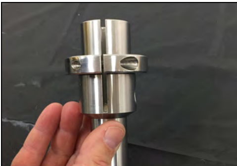
Figure 81 - Slide shaft collar on stub shaft
