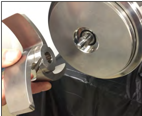
Figure 107 - Install impeller on stub shaft
