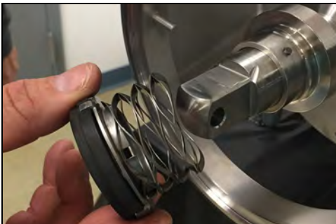
Figure 19 - Remove seal, O-ring, seal cup and spring
