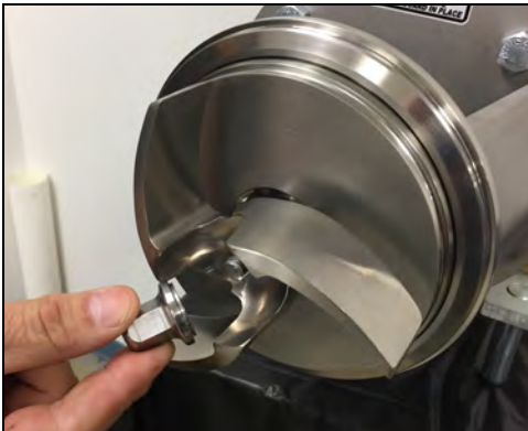
Figure 89 - Install impeller nut
