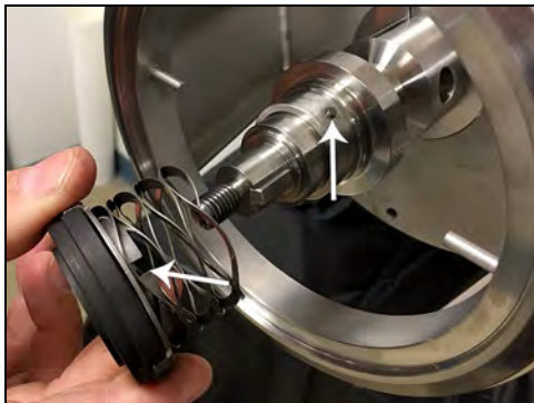
Figure 98 - Line up groove and pin
