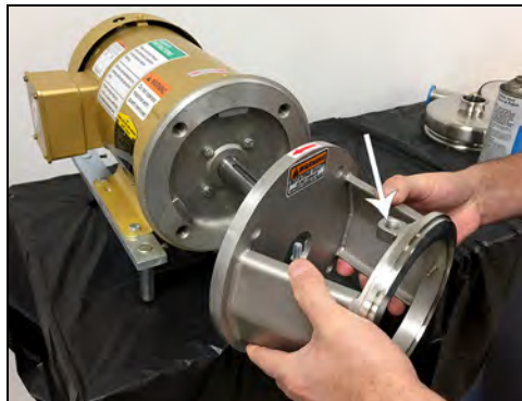
Figure 77 - Install motor adapter
