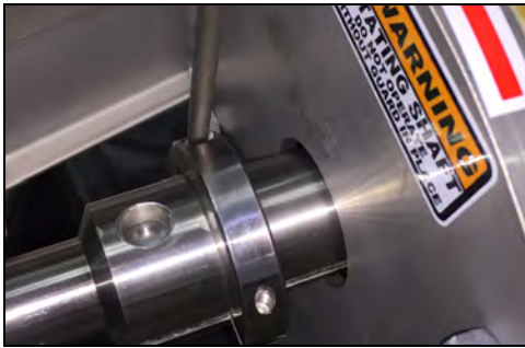
Figure 72 - Loosen shaft collar screws
