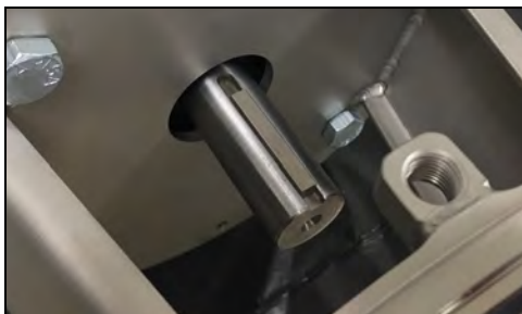
Figure 29 - Install key in motor shaft
