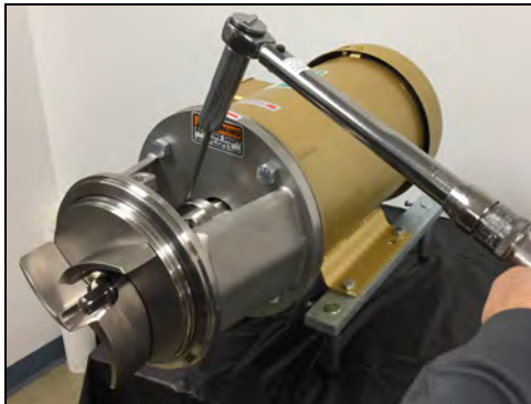
Figure 92 - Torque shaft collar screws
