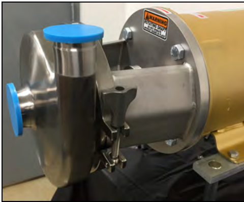
Figure 116 - Hand-tighten casing clamp
