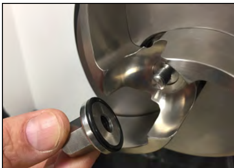
Figure 61 - Remove impeller nut
