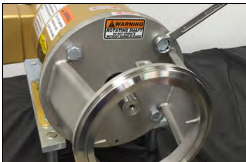
Figure 28 - Install motor adapter bolts
