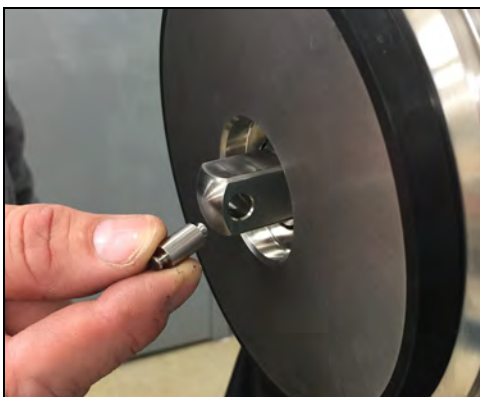
Figure 33 - Insert impeller retainer pin
