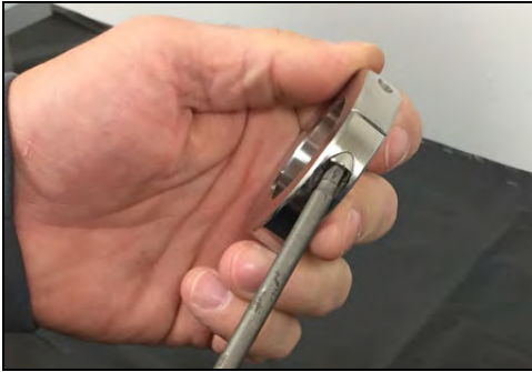
Figure 79 - Remove shaft collar screws
