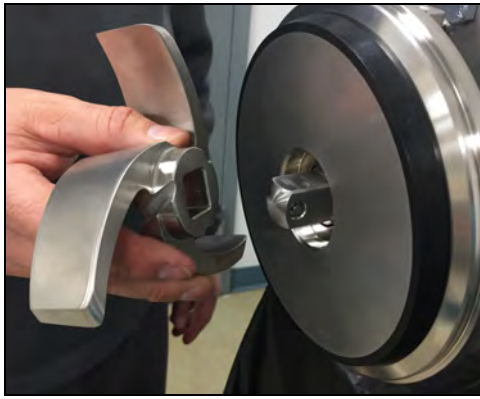
Figure 35 - Slide impeller on shaft
