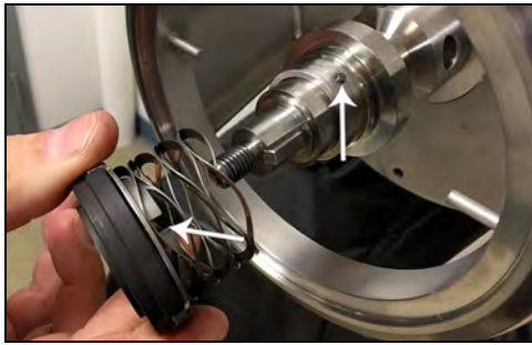
Figure 66 - Remove seal, cup, and spring
