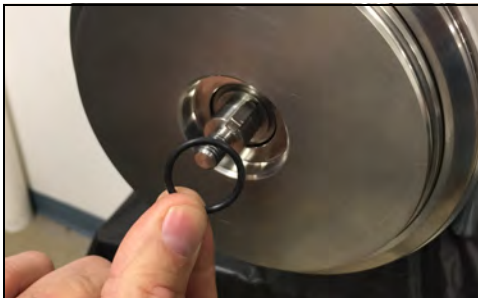
Figure 64 - Remove stub shaft O-ring
