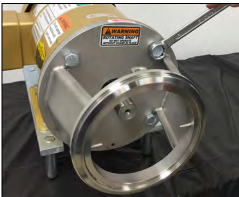
Figure 74 - Remove motor adapter bolts
