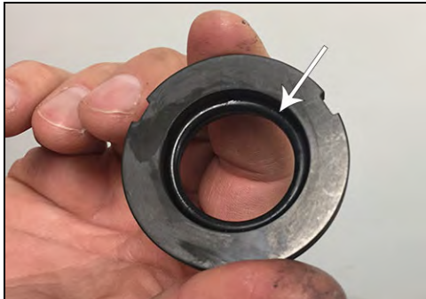
Figure 97 - Seal O-ring installed
