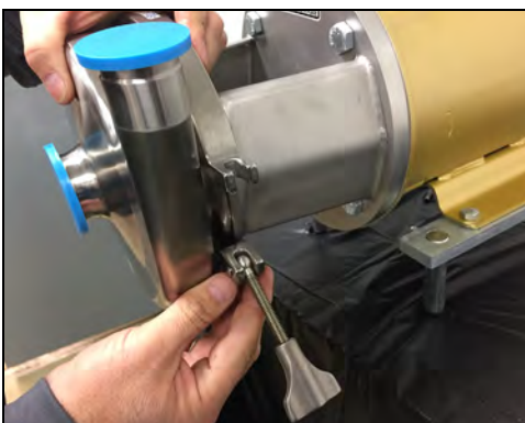
Figure 115 - Install casing clamp
