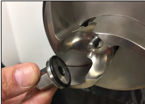
Figure 109 - Install impeller nut
