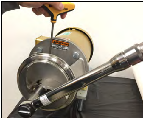
Figure 60 - Loosen impeller nut
