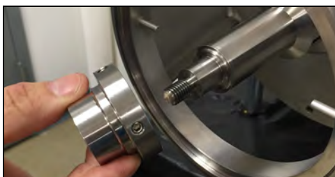
Figure 71 - Remove drive collar
