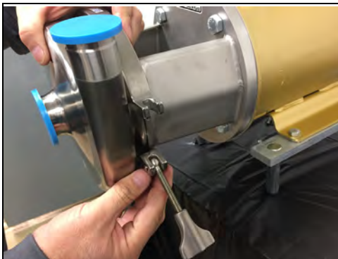
Figure 12 - Remove casing clamp
