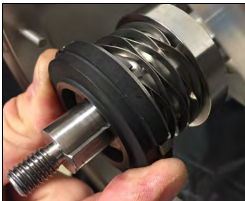
Figure 99 - Push seal on stub shaft
