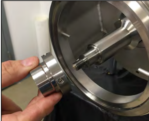
Figure 93 - Place drive collar on stub shaft
