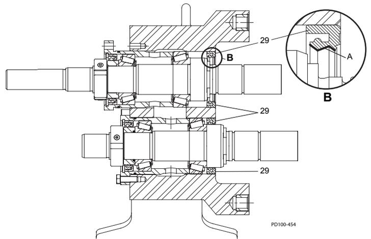
Figure 48 - Apply Bearing Grease
