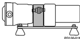
Figure 6 - Leveling and/or Vibration Isolation Pads
