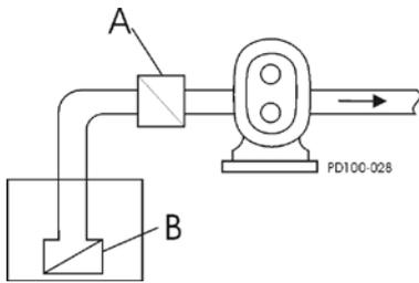
Figure 12 - Inlet Check Valve
