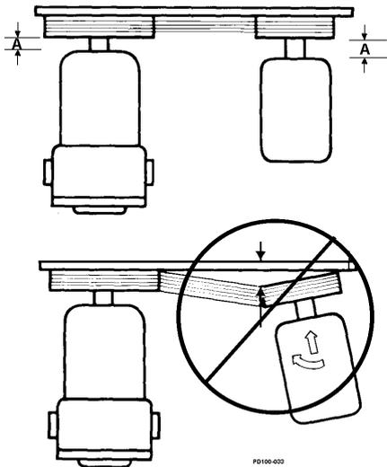
Figure 21 - Alignment Belt and Chain Drives
